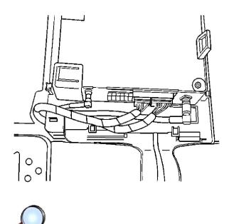
2. Install the module to the upper bracket ensuring the retaining tab is fully seated.
